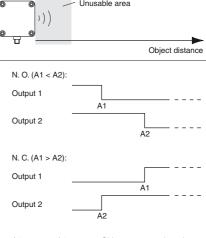
A1→ ∞ , A2→ ∞ : Object presence detection Both outputs are active if Object within detection range.
