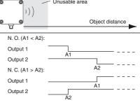
A1 → ∞, A2 → ∞: Object presence detection Both outputs are active if Object within detection range.
