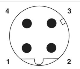
Pin assignment M12 male connector, 4-pos., D-coded, male side
