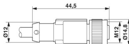
M12 x 1 female connector, straight, shielded
